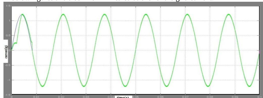
Fig.6.17: Grid current i_g and its reference i_{g-ref} when the PR controller with fuzzy logic controller is applied
