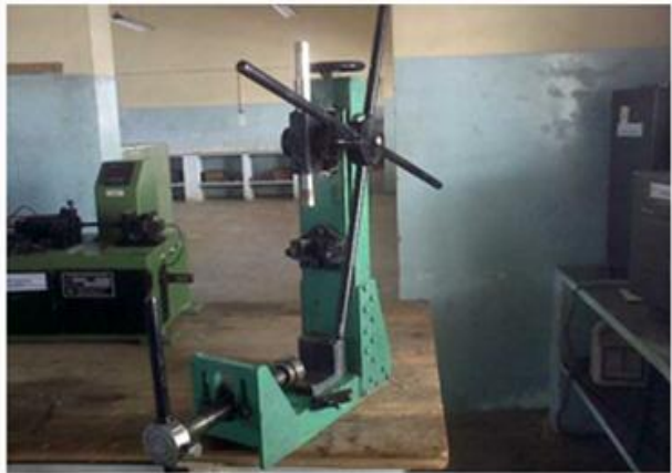
Fig. 2 Image of the injection molding machine used in this study
