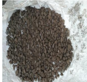
Fig 2. Fly Ash Coarse Aggregate of 20 mm Size
