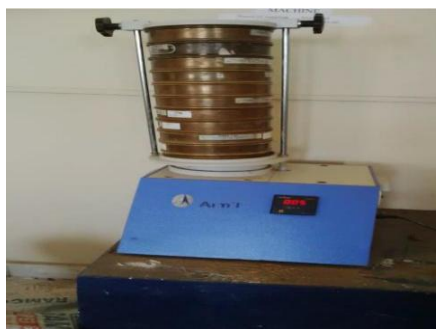
Figure 5: Showing the Sieve Analysis For River Sand
