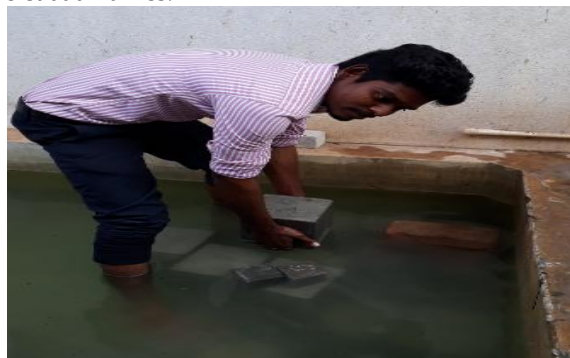
Figure 13: Showing the Curing Of Specimens
