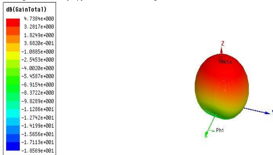
Fig. 7 Polar plot of planar antenna with Rogers RT duroid 5880 as a substrate.
