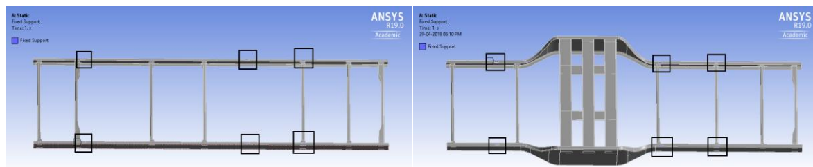
Fig. 7: Fixed-Fixed modal analysis constraints on frames
