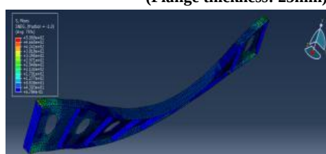
Von Mises Stress Distribution
