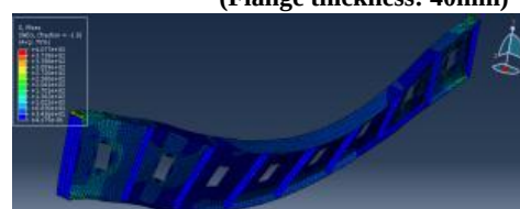
Von Mises Stress Distribution
