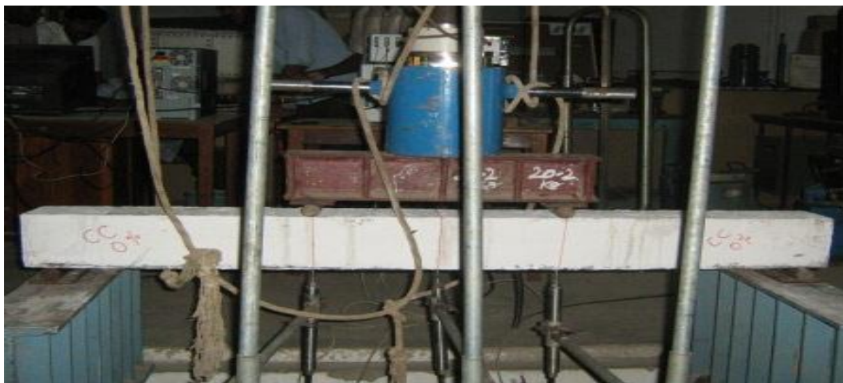
Fig 6: Experimental Setup of RCC beam
