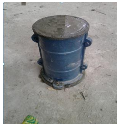
Fig 3: Casting of Cylinders
