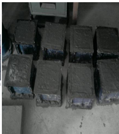
Fig 2: Casting of Cubes
