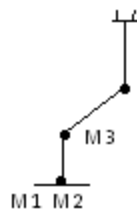
Fig.2.3 3R Structure 2 e_{21}=1, e_{31}=0 e_{32}=1, t_{21}=-1 t_{31}=1, t_{32}=-1
