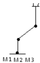
Fig.2.2 3R Structure 1 e_{21}=1, e_{31}=1 e_{32}=1, t_{21}=-1 t_{31}=0, t_{32}=-1
