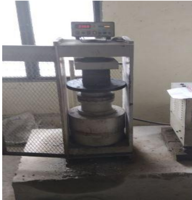
Figure 1: Compressive testing machine with setup
