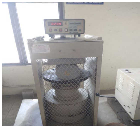
Figure 2: Compressive testing machine with setup
