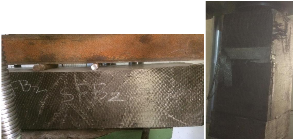
Fig 7. Failure behaviour of beam and column
