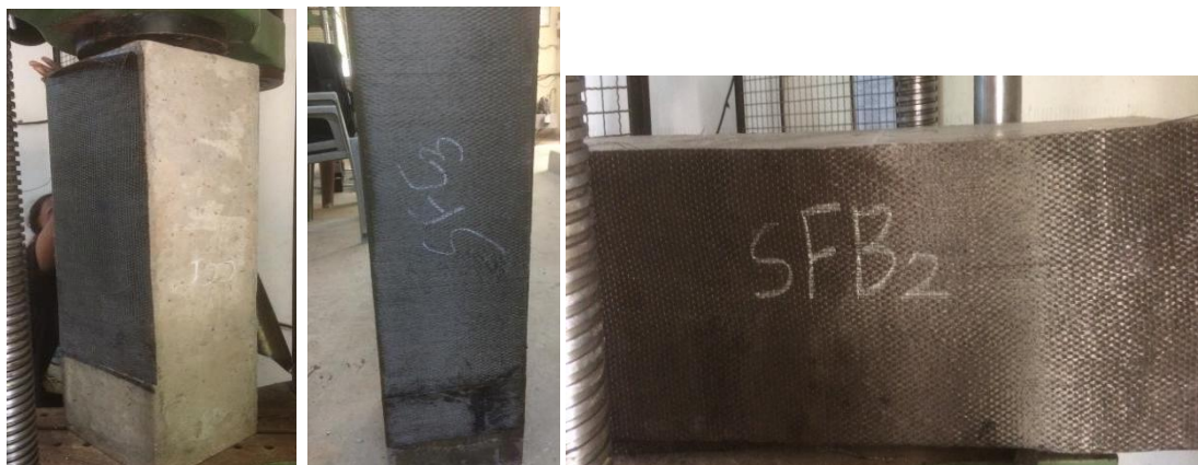
Fig.4 strengthening of column and beam
