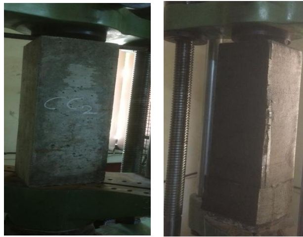
Fig. 3 Test set up of with and without strengthening of column
