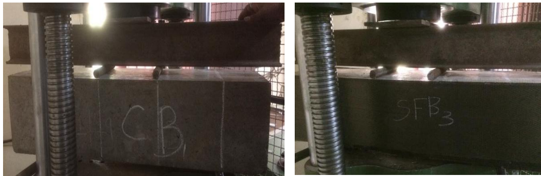
Fig. 2 Test set up of with and without strengthening of beam
