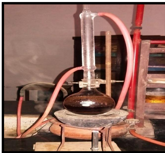
Fig. 2. Photograph of Experimental Setup for Obtaining Grevillea robusta Leaf Extract Using Reflux Condenser
