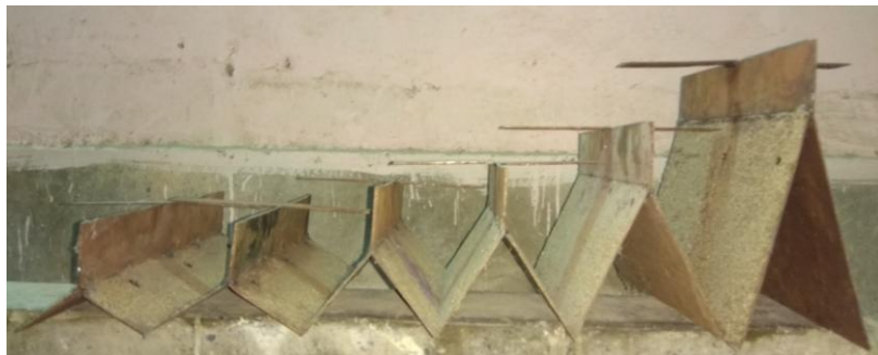
Fig. 2. Upright Model Shell Footing used for Experimental investigation
