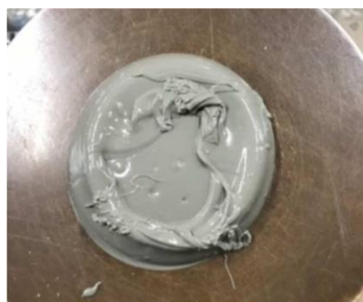
(a) Lift the mold away from the paste
